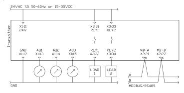
Relay contact rating is max. 1A at 230 VAC
