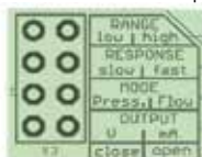
Volume flow mode: Jumper 3 open
